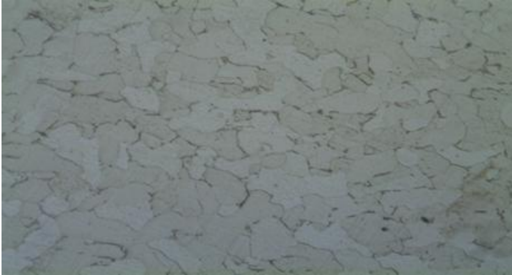
Figure 3. Typical Microstructure of the ASTM A1011 steel sheets (X50)
