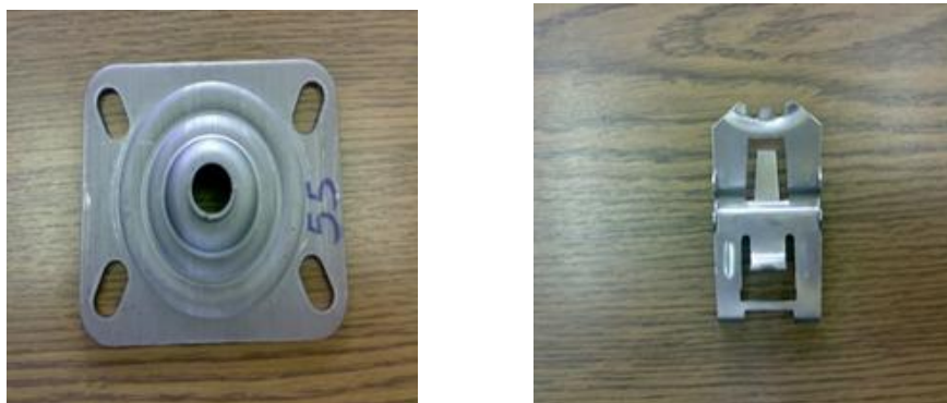
Figure 2. Studied products of ASTM A1011 sheets for garbage container wheel parts
