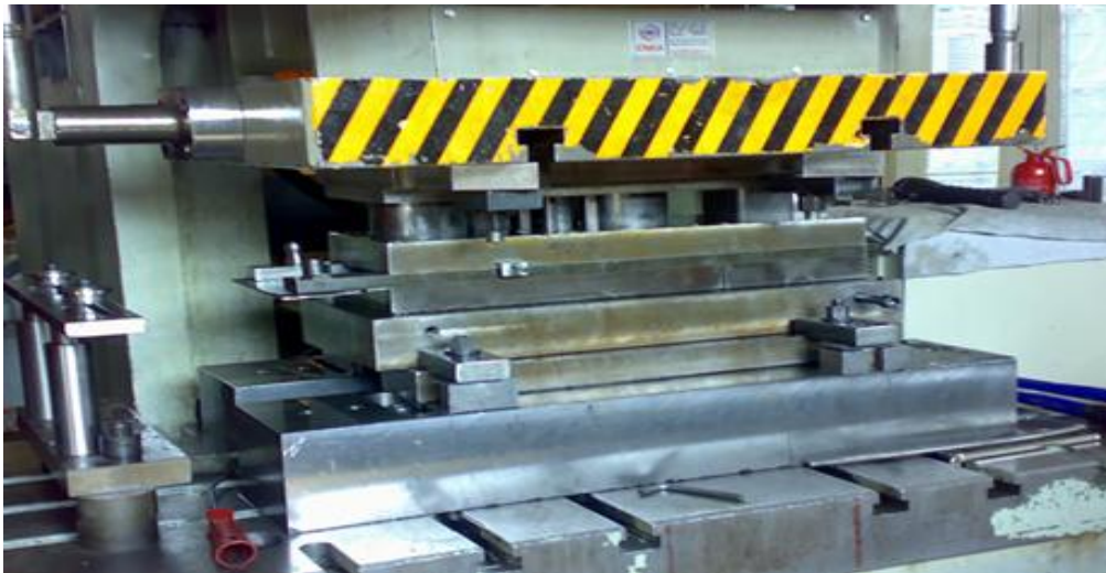
Figure 4. Punch press and sheet metal blanking process
