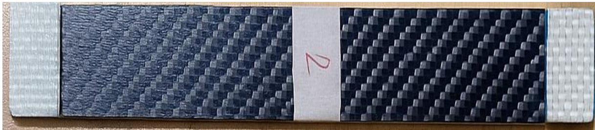
Figure 1. The composite specimen with twill pattern prepared for tensile test
