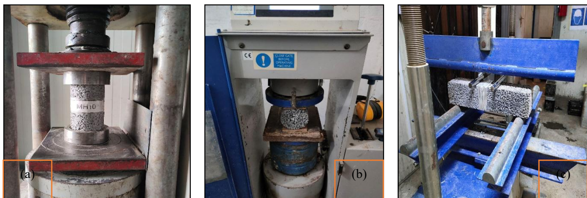
Figure 2. The performed tests: (a) compression resistance, (b) tensile splitting strength, and (c) flexural strength
