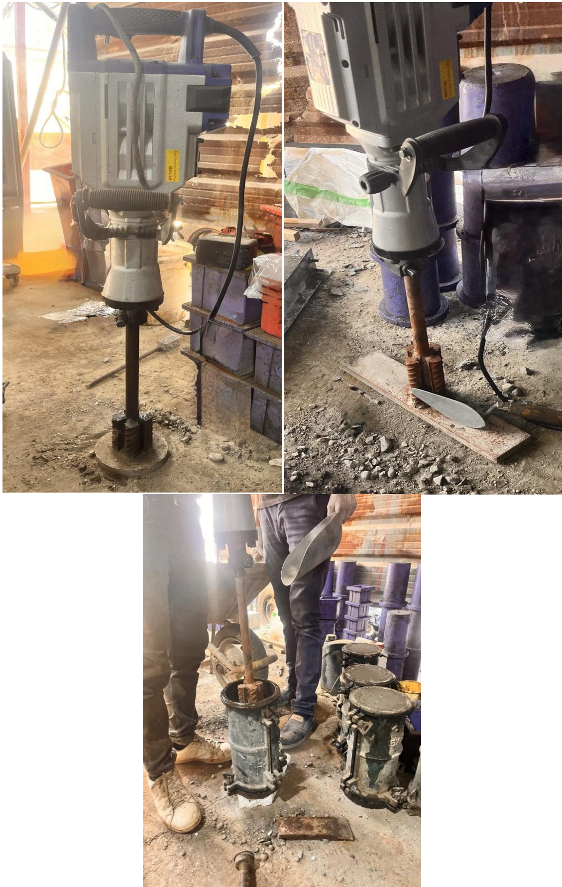
Figure 5. The vibrating hammer with a tamping plate
