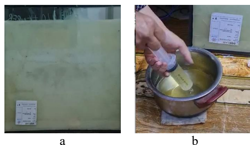
Figure 3. (a) Window with integrated PCM. (b) Injecting liquid PCM into the double-glazed cavity.
