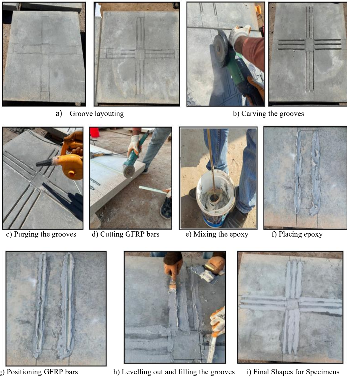
Figure 4. Strengthening procedure of the RC slab specimens
