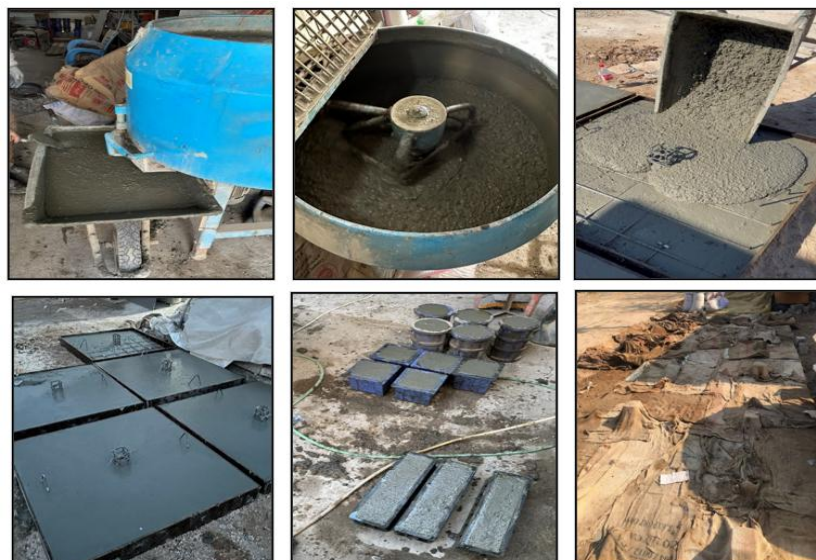
Figure 2. Casting and curing the RC slab specimens, cubes, cylinders and prisms.
