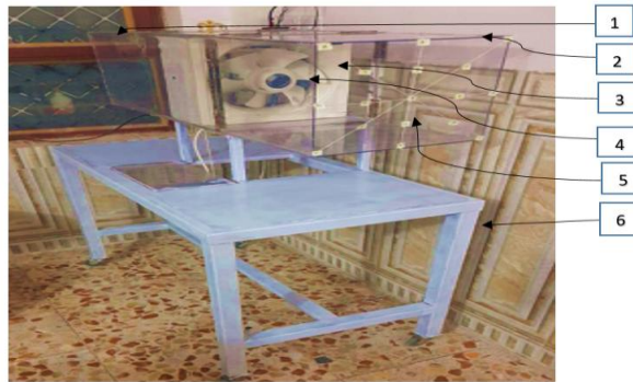
Figure 1. Experimental setup device. (1-outlet 2- plastic glass 3- shroud 4- axial fan 5- inlet 6- Iron scale)
