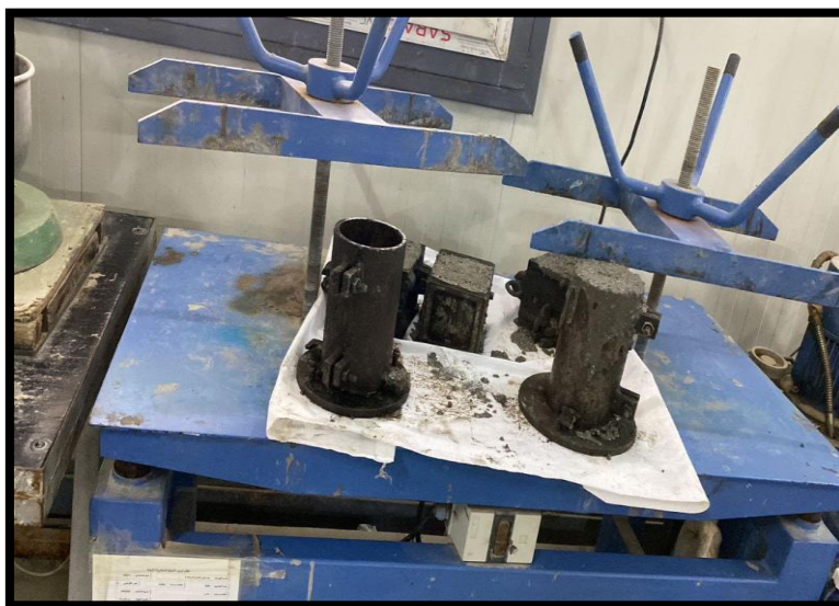
Figure 3. Compaction of the tested mixes
