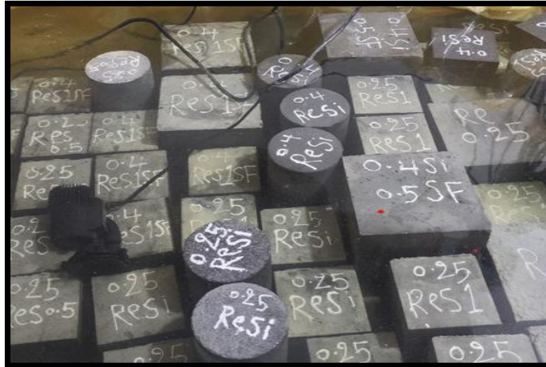
Figure 4. Curing of the prepared HSLWC
