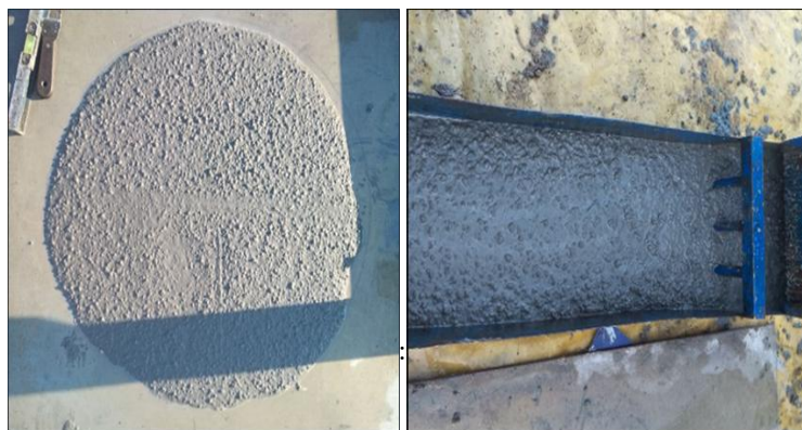
Figure 4. Fresh tests of LWSCC: spread slump flow and L-box tests
