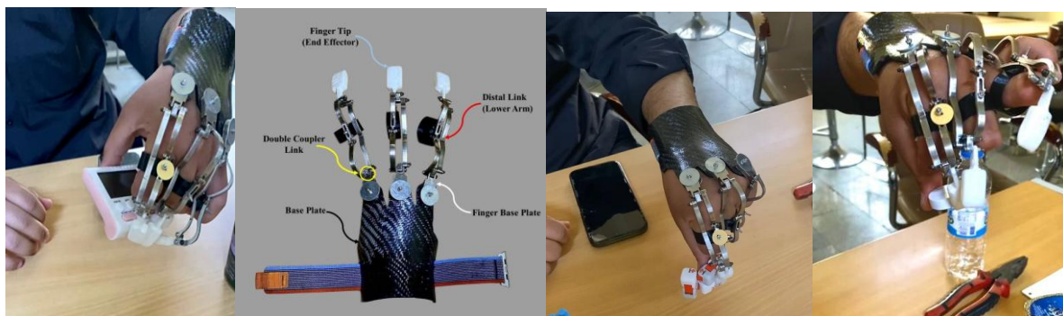
Figure 5. Application of standardized hand function tests (Jebsen–Taylor & Box and Block) on the fabricated prosthesis
