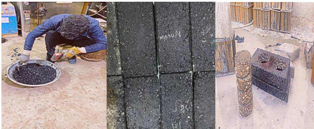
Figure 8. Conducting the (WTT) to evaluate the performance of modified asphalt mixtures
