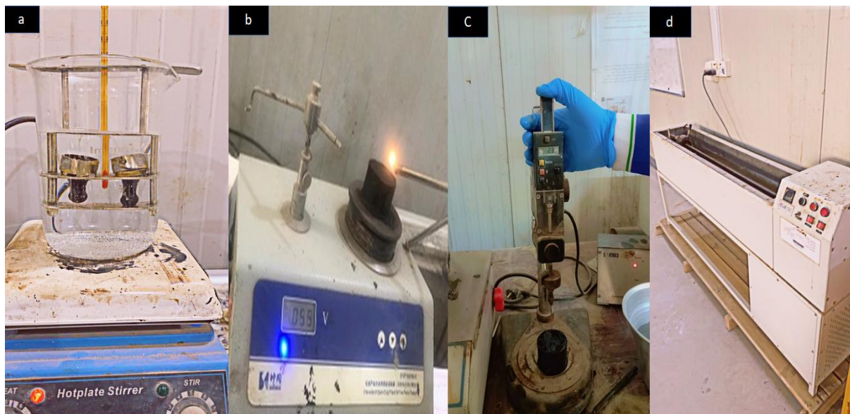
Figure 2. Asphalt test: (a) Softening point, (b) Flashpoint, (c) Penetration, (d) Ductility
