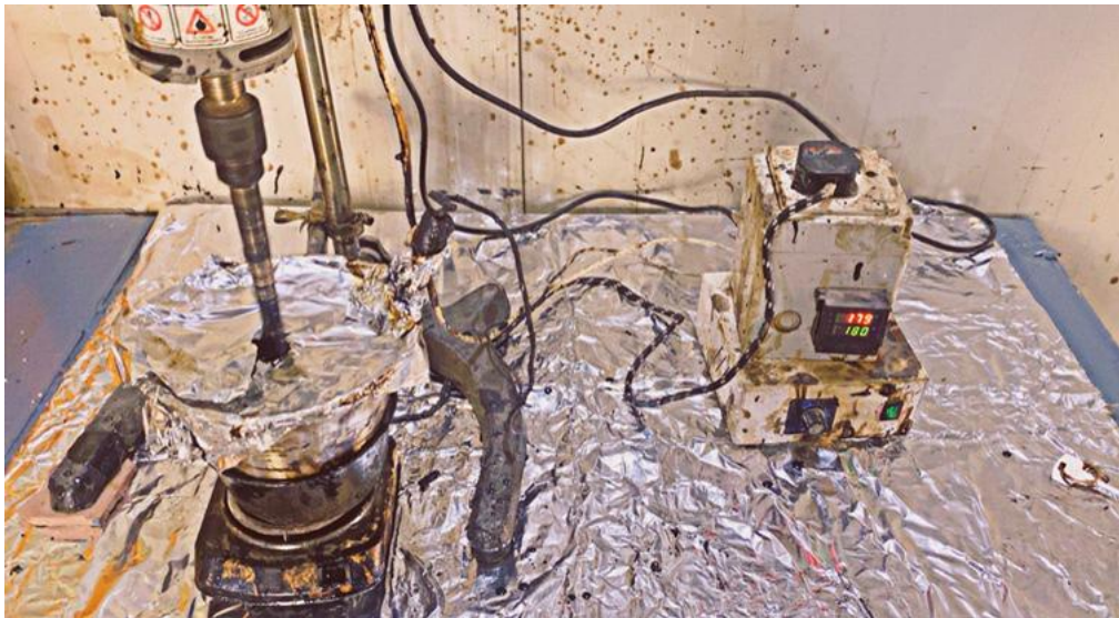
Figure 4. Preparation of polymer blend to enhance bitumen properties
