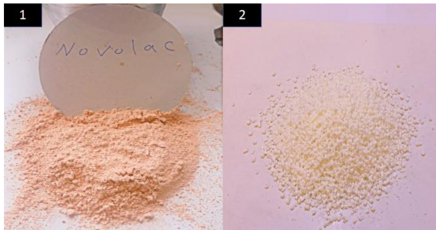
Figure 3. Physical forms of asphalt modifiers: (1) Novolac powder and (2) SBS granules
