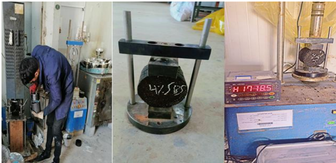
Figure 7. Laboratory tests of ITS devices and specimens at the University of - Al- Qadisiyah
