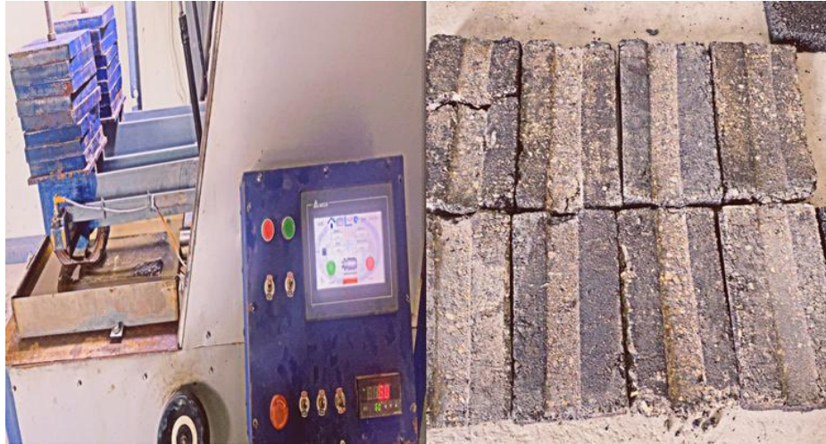
Figure 17. Effect of rut depth under wheel tracking test on asphalt samples
