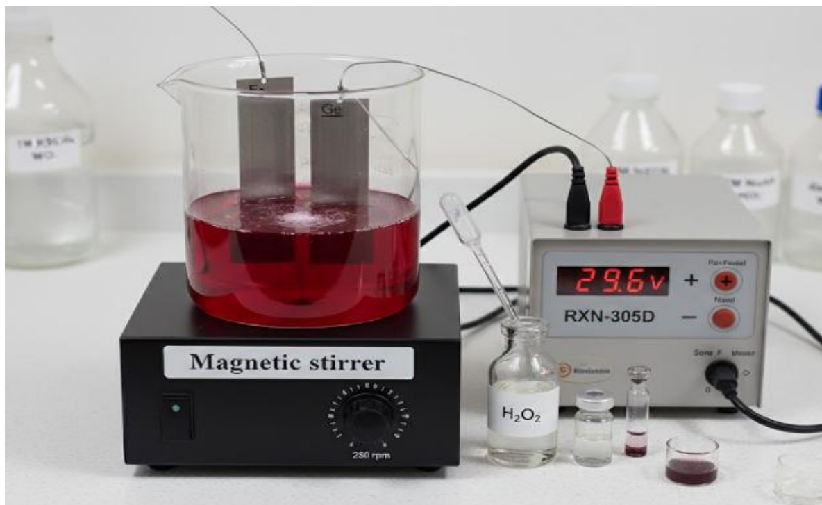
Figure 2. The electro-oxidation reactor scheme.
