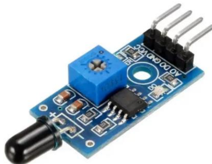
Figure 4. REES52 IR flame sensor
