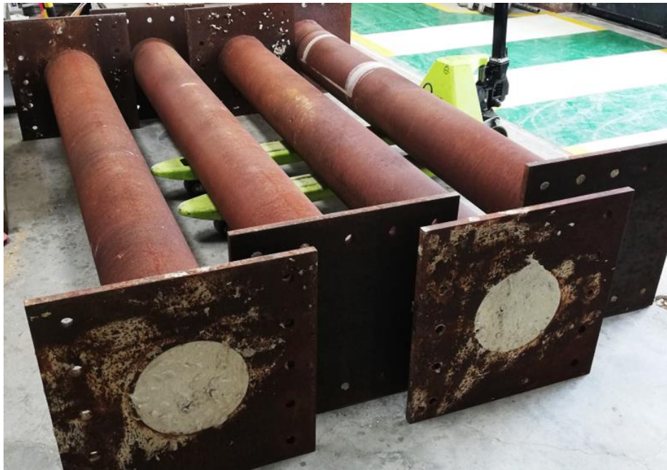
Figure 3. C5-C8 CFT specimens.
