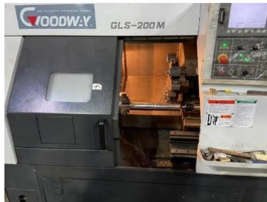
Figure 1. CNC Lathe Machine GLS-200 M
