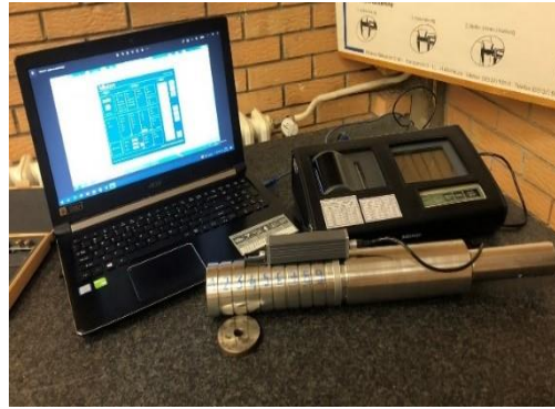
Figure 3. Surface roughness measurements with Mitutoyo SJ-310
