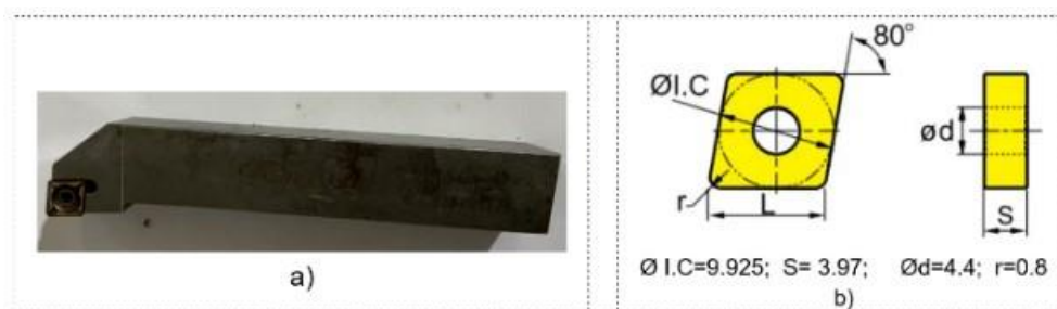
Figure 2. a) Toolholder SCLCR 2020 K89 – Techno Takim, b) Cutting insert CCMT 09T308N
