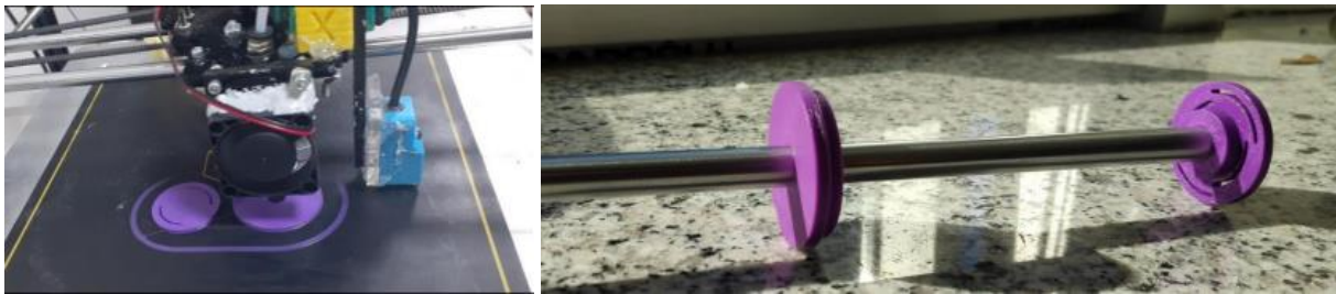
Figure 2. Shock absorber parts produced with 3D printer
