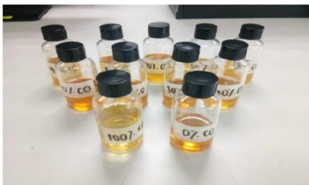
Figure 1. View inspection (Change in engine oil color against the composition percentage)
