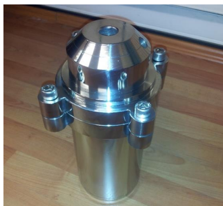
Figure 2. Photograph of designed and manufactured supercritical reactor.
