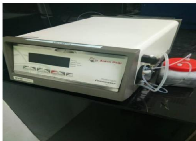
Figure 2. The 2 nd generation stabinger viscometer 3000 (SVM 3000/G2)
