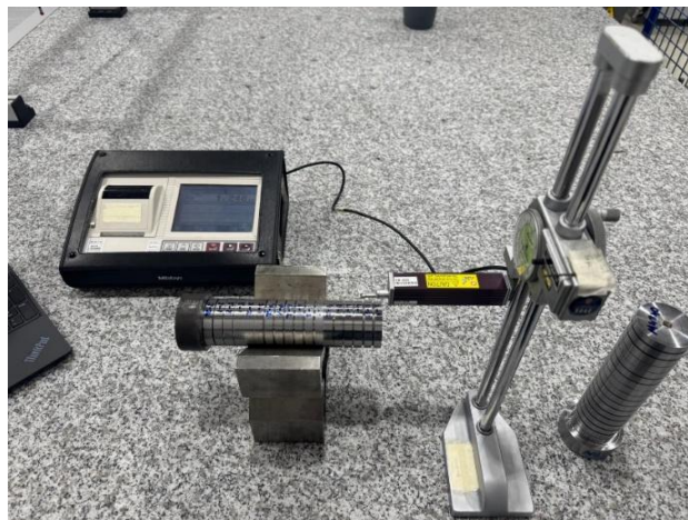
Figure 3. Fixed surface-roughness surface measurement system, and to be measured specimen
