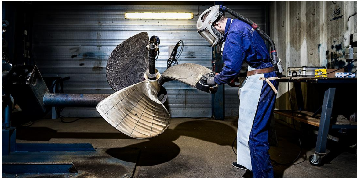
Figure 1. 3D printed ship propeller (Ship- shape)
